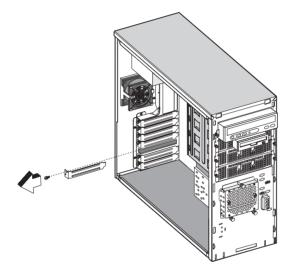
3 Insert an expansion card into the slot. Make sure that the card is properly seated.
